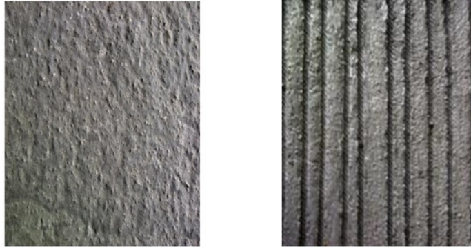
Figure 1. Difference of substrate surface conditions between as-placed and longitudinally roughened with 6 mm of roughness amplitude
