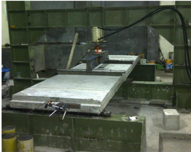
Figure 3 Flexural test setup of the composite concrete slab
